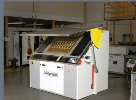
Pneumatic lifting of frames
